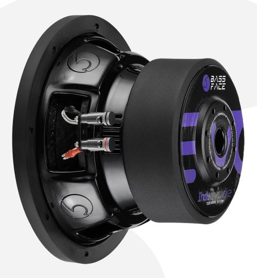
Every subwoofer installation needs a crossover function - the precise settings are a subject of discussion for each particular setup but a good starting point is to work with a 25Hz subsonic (high pass) filter and a 100Hz low pass filter. Whilst these will not produce optimum results in every case they will certainly be enough to get you up and running.
