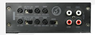
Time to lay on some power. Connect the earth first, then 12V power, then remote. Then connect in the RCA cables and you can move onto setting up sound controls on the amplifier. This description covers the principles of operation – for specific instructions refer to the set up notes for the exact model you are working with.
